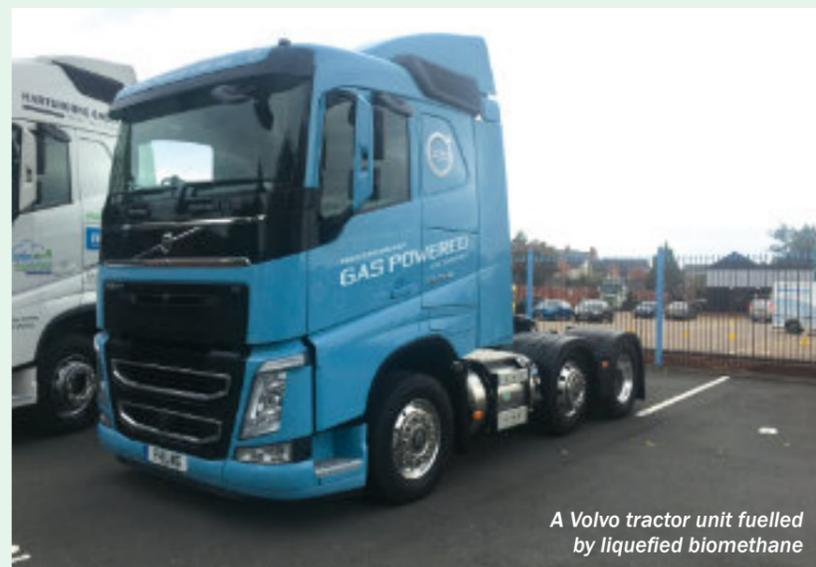
A Volvo tractor unit fuelled by liquefied biomethane
