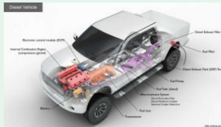
Biodiesel and conventional diesel vehicles are essentially one and the same. Although light-, medium-, and heavy-duty diesel vehicles are not technically alternative fuel vehicles, almost all are capable of running on biodiesel blends (always check before use).
