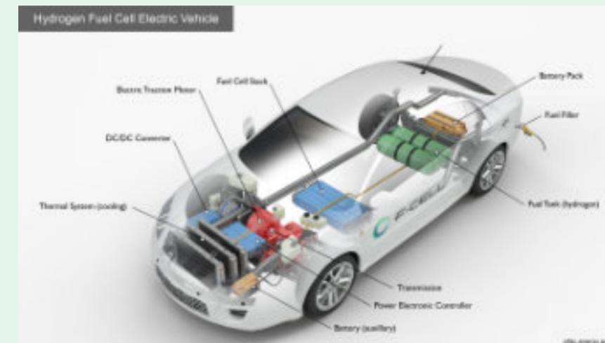
Energy is stored as hydrogen in a tank on the vehicle and then converted to electricity by the fuel cell. Unlike conventional internal combustion engine vehicles, these vehicles produce no harmful tailpipe emissions, only emitting water vapour and air. They can be refuelled quickly and have a potential driving range over 300 miles.
