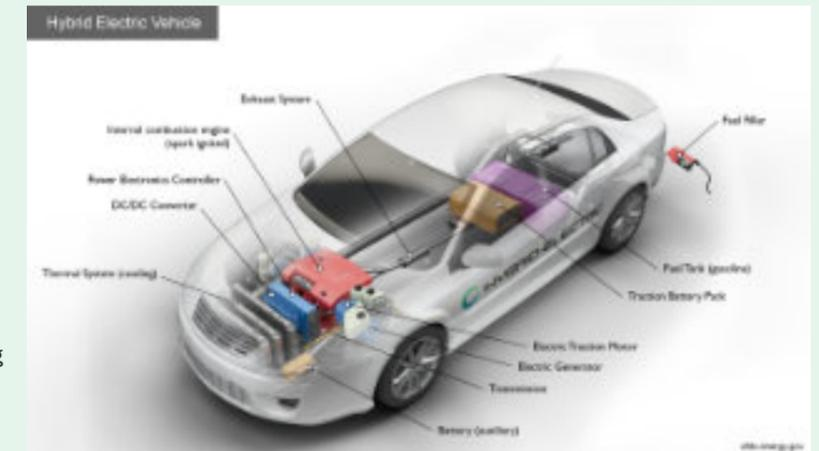
The vehicle uses regenerative braking and the internal combustion engine to charge. It captures energy normally lost during braking, by using the electric motor as a generator and storing the captured energy in the battery.
